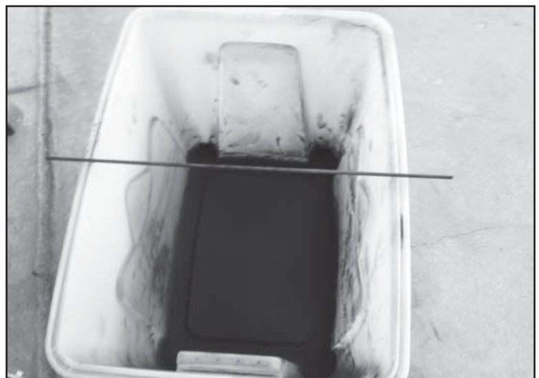
A plastic container (15-quart size or larger, serving as the storage container for powder coating system components) may serve as a portable “spray booth.”
